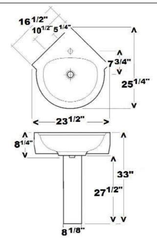
Dimensions of fixture are nominal and may vary within the range of tolerances established by ASMEI Standard A112.19.2-2018. Dimensions and specifications subject to change without notice.
